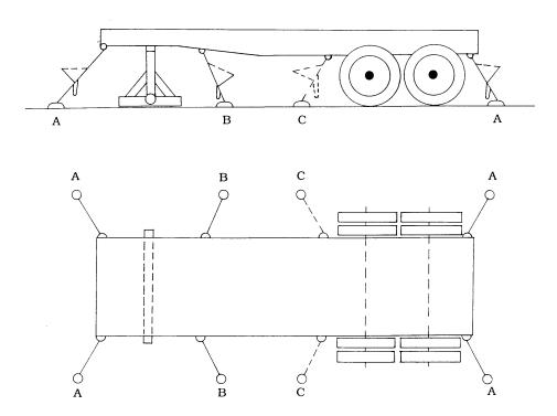
Trailers and similar road vehicles must comply with the specifications in respect of Lashing and Securing arrangements on road vehicles for sea transportation on ro-ro ships. In this respect we are referring to the International Standard ISO 9367-1 and ISO 9367-2 and the specifications as Described in the IMO Resolution A581 (14).
